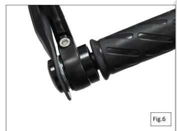
6. Fit the hand guards to the brackets using M6 x 20 flange screws (5) and M6 Flange nut (3) inside hand guards as shown in Fig 7. Tighten bar end screws.
